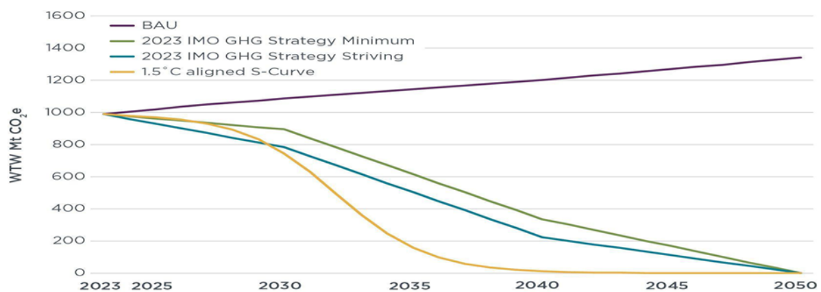
Absolute well-to-wake GHG emissions trajectories under each scenario vs business as usual scenario (Carvalho & Comer, 2024)
