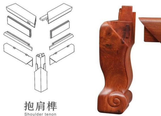
Figure 1. Comparative Visualisation of Shoulder Tenon
