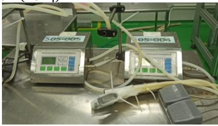
FIGURE 1. CNC filling machine (old filling machine).
