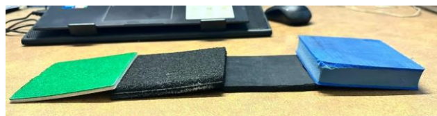
FIGURE 4. Result of the rubber material after undergoing the cutting process in required temperature.
