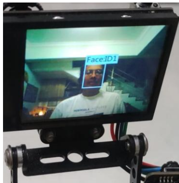
FIGURE 8. The robot detected a recognized face.
