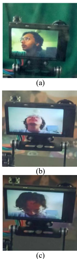
FIGURE 10. HUSKYLENS unable to recognize faces pointed (a) sideways (b) upwards (c) downwards.
