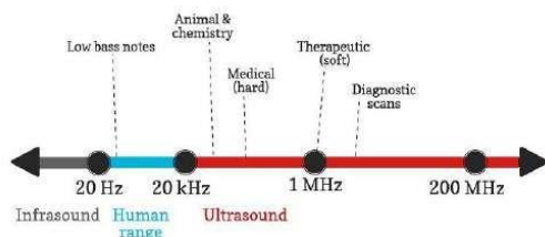
FIGURE 1. The operating frequencies for typical applications of ultrasonic waves [35].
