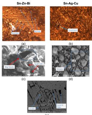
FIGURE 2. Optical and SEM micrographs of solder joint fracture surfaces (a) Sn-3Zn-4Bi fracture surface under OM (20×) (b) Sn-Ag-Cu fracture surface under OM (20×) (c) SEM image of Sn-3Zn-4Bi fracture surface showing voids and microstructural features (d) SEM image of Sn-Ag-Cu fracture surface with smoother morphology (e) SEM micrograph of Sn-3Zn-4Bi bulk solder revealing grain structure and phase distribution.
