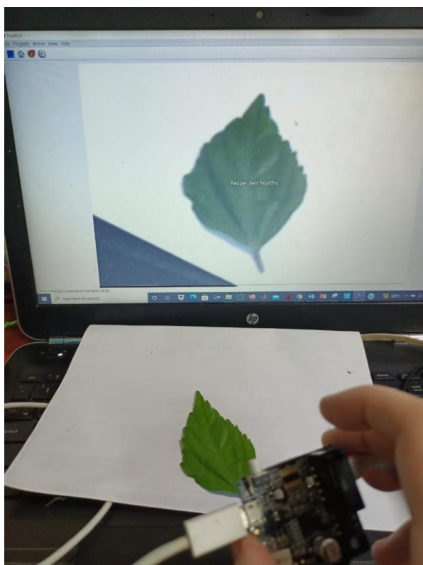
FIGURE 7. Camera system with CNN model for detecting and classifying plant diseases.
