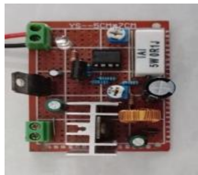
FIGURE 6(C). The combined circuit of buck converter and current limiter.
