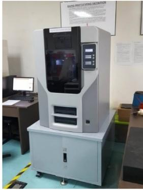
Fig. 1. Dimension SST 1200es Rapid Prototyping Machine.
