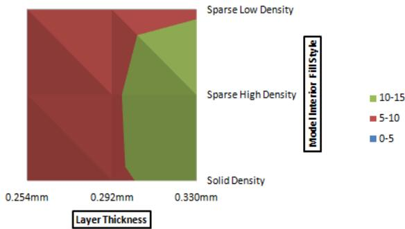
Fig. 3. Contour graph of surface roughness.
