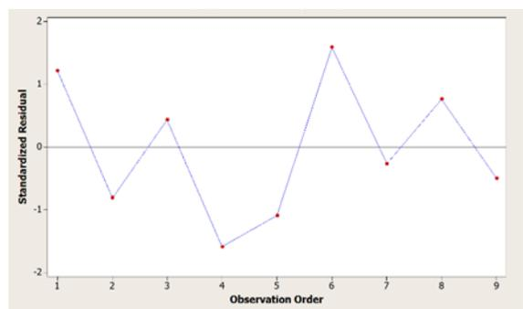
Fig. 7. Residual versus order chart of the surface roughness.
