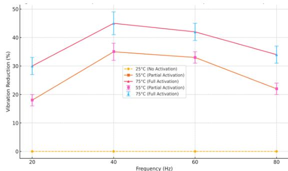
Fig. 2. Vibration amplitude before and after SMA activation at different temperatures and frequencies.
