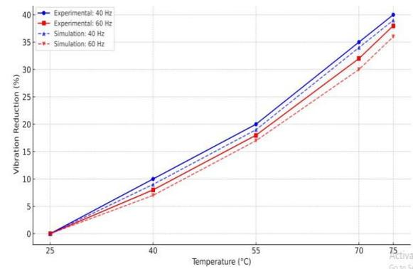
Fig. 3. Vibration amplitude reduction as a function of temperature for 40 Hz and 60 Hz.
