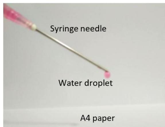
Fig. 1. Wettability test of a water droplet on the tested paper.
