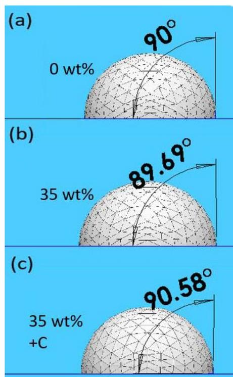
Fig. 3. Wettability condition of water droplet on Sand/HDPE sheet (a) 0 wt% composite (b) 35 wt% composite (c) 35 wt% + C composite.
