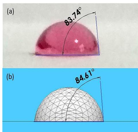
Fig. 2. (a) Contact angle of droplet on the tested paper obtained from the current experimental study (b) Contact angle from the current modelling result on the tested paper using Surface Evolver.
