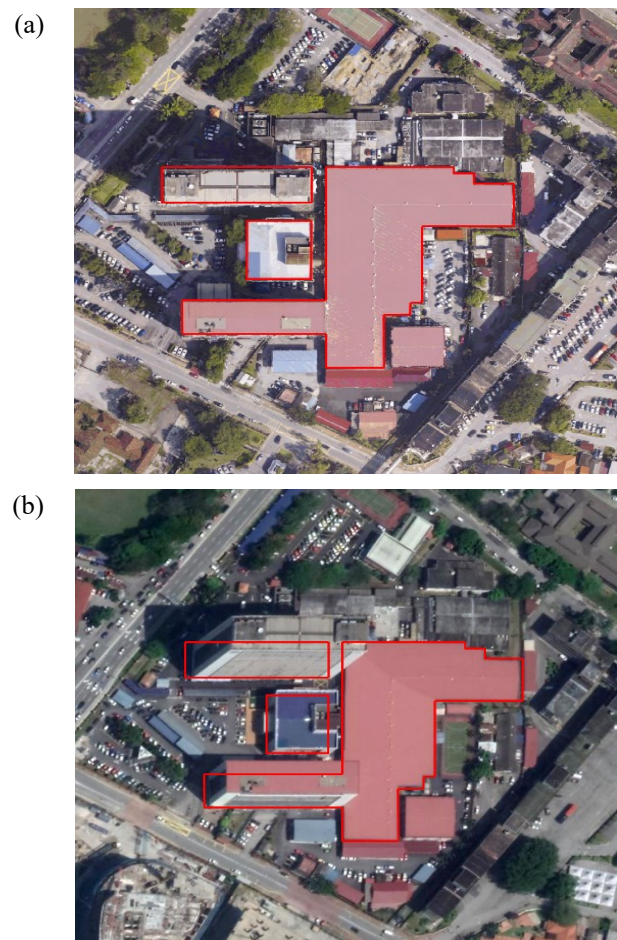
Fig. 6. Different between (a) true-orthophoto and (b) orthophoto imagery.
