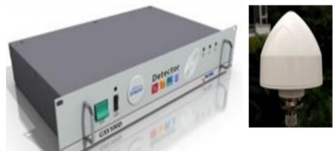
Fig. 2. Detector V1 and GNSS L1 receiver used in the study.
