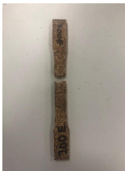
Fig. 2. The fractured tensile test sample.
