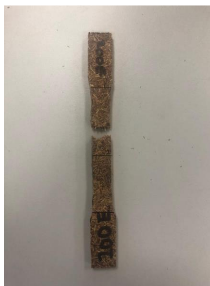
Fig. 2. The fractured tensile test sample.
