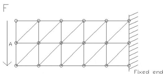
Fig. 1. A deep cantilever beam with point load.
