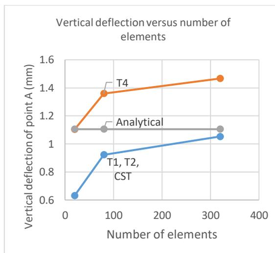
Fig. 2. Simulation results for constant strain functions.
